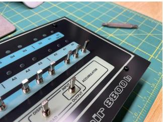
This will provide the optimum spacing for the toggles. Turn the board over and solder the toggles.
