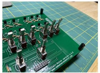
Put the toggles in place, then put the front panel in place and secure with 10mm nylon screws.
