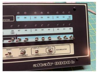
Now turn the whole assembly over and make sure the LEDs are seated in the holes cut in the spacer and resting on the back of the front panel. Solder the LEDs in place.
