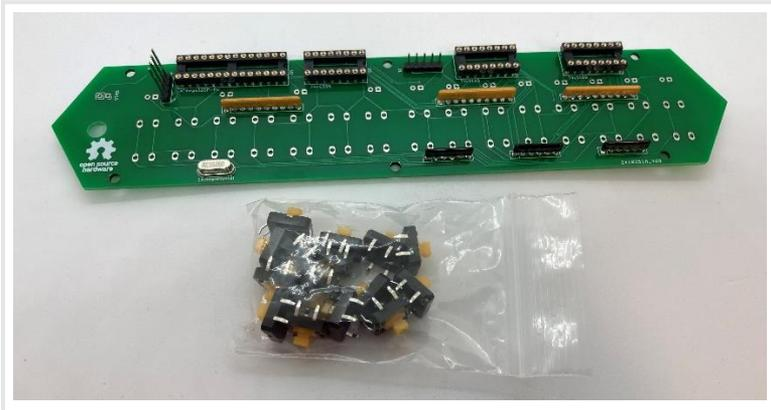
These will be placed on the front side of the circuit board (with the Adwater & Stir logo.) It is important that they are installed flat and aligned, so they will later align correctly with the front panel.
