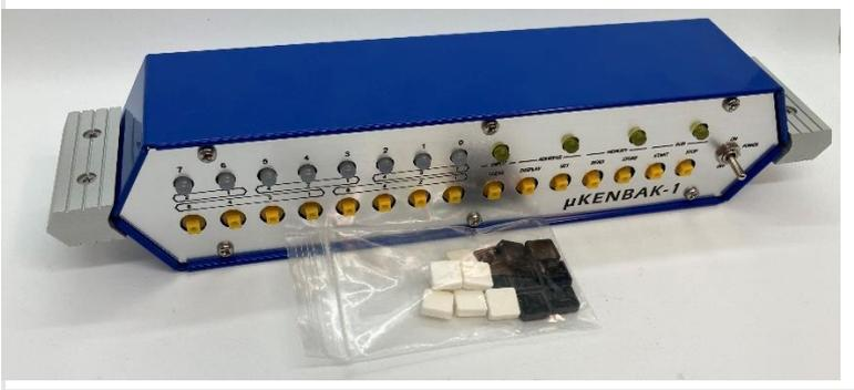
The button caps will fit in any orientation, but I have found that it's best to have the buttons mounted as pictured. It makes it easier to pry the buttons off (from the top and bottom) if necessary.
