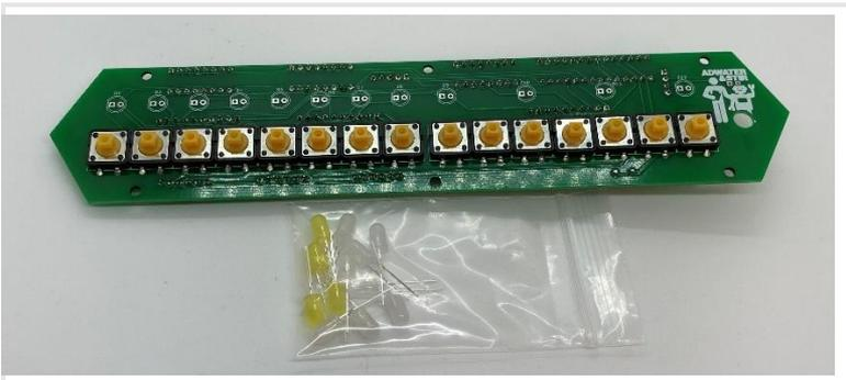
The orientation of the LEDs is crucial. Make sure the long lead of the LED is toward the right of the PCB and the flat side of the LED is toward the left (as indicated on the screen print.)
