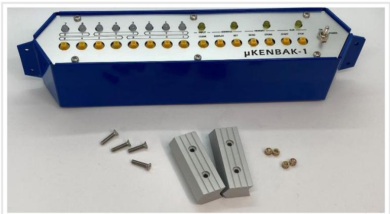
The pieces are held in place by 14mm flat head bolts and brass knurled nuts.
