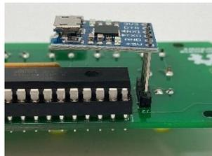
This is a good time to check the function of your kit. You can plug a micro USB cable into the USB to UART module, flip the power switch up, and the  $\mu$ Kenbak-1 should be fully functional.
