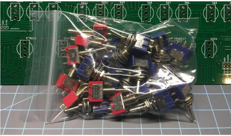
Put all the switches in place *without soldering them*. 17 two position toggles on the top row and the power switch location, 8 three position momentary toggles on the bottom row.
