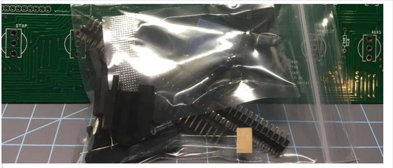
In that bag you will find one electrolytic capacitor and one  $470\Omega$  resistor (Yellow, Violet, Brown, Gold color code). If you don't want to decipher the color code, just know you will find three resistors in the bag, two that match, and one that does not. This is the one that does not match another.
