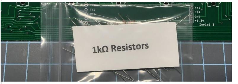
Add the 36-1k $\Omega$  resistors to the top rows under the LED/Transistor pairs in locations R1-R36. Resistors are non-polarized, meaning they can go in either direction; you do not need to worry about orientation.
