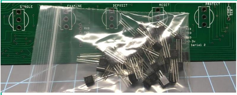
The orientation of the transistor is crucial, but relatively simple. Just make sure the flat end of the transistor is facing up, just like the image printed on the circuit board.
