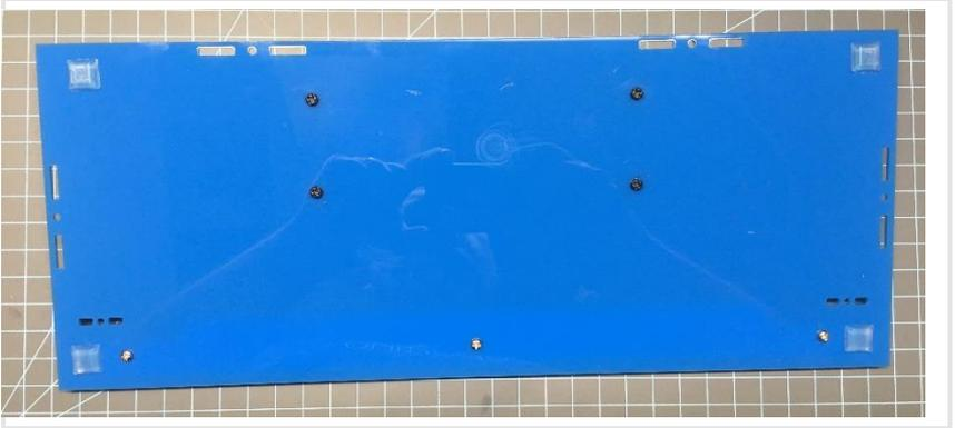
Next we're going to start joining acrylic pieces with a t-slot joint. Start with the uprights where we will eventually mount the main circuit board. Attach them to the bottom piece with 14mm bolts and square nuts. Tighten firmly, but not too tight – acrylic can crack.
