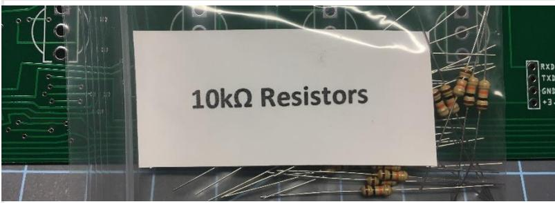
Add the 36-10k $\Omega$  resistors to the second row in R37-R72.
