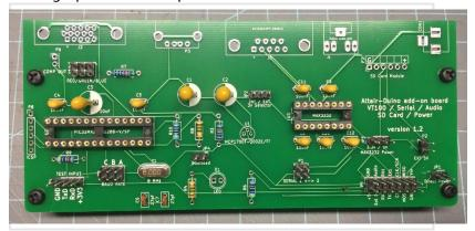
Add the LED (with long lead to the right and flat side to the left) and the MCP1700 voltage regulator with the flat side down.
