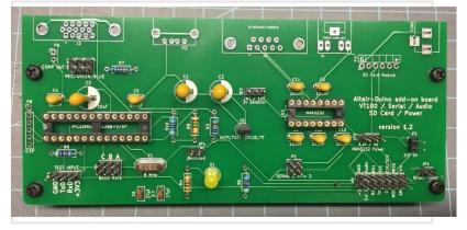
Version 1.3 of the board now includes a 5v voltage regulator (to allow use of a power adapter 9v-12v). Add the LM7805 regulator, 100nF capacitor, and 10uF capacitor to this location:
