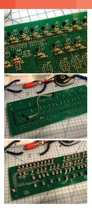
LIGHTS, SWITCHES, ACTION: A printed circuit board contains additional circuitry for driving LEDs [top], but most of the work is handed off to an Arduino Due plugged into a rear connector [middle]. The finished PCB [bottom] is mounted in the case.
