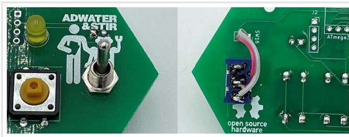
This is a good time to check the function of your kit. You can plug a micro USB cable into the USB to UART module, flip the power switch up, and the  $\mu$ Kenbak-1 should be fully functional.
