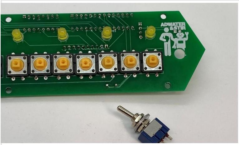
Remove the nuts and washers from the switch, secure it in place with a single nut, then turn the board over and solder a wire from SW16 to the center pin and bottom pin on the switch, as pictured.
