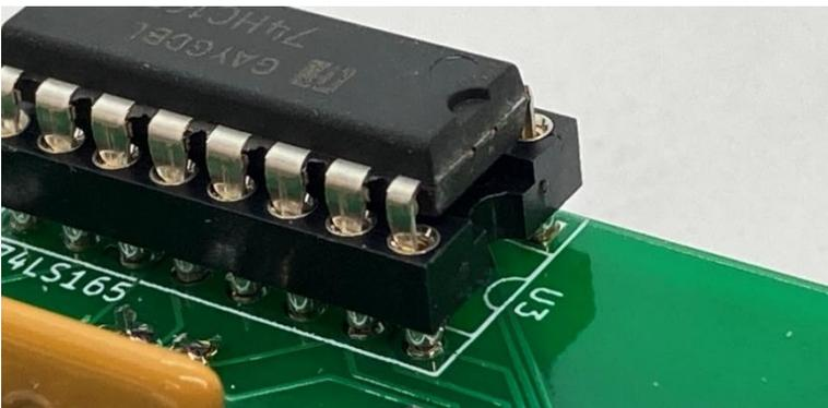
Note that there are two 74LS165, and one 74LS595. Make sure they are installed in the correct sockets as labeled on the circuit board.
