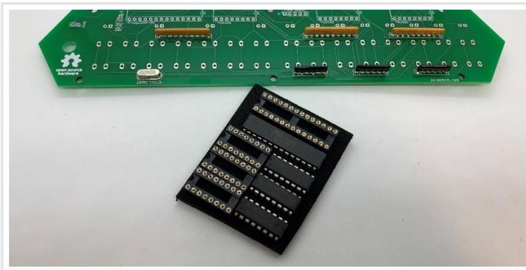
Make sure the DIP sockets are mounted with the notch facing right as indicated by the screen printing on the circuit board.
