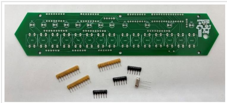
The 6-pin black resistor arrays are 10k $\Omega$  and the orientation is important. They are installed in RN2, RN3, and RN6. The end with the white dot should be installed in the square pad on the left side:
