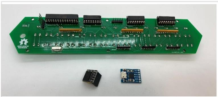
The DS3231 module simply mounts on the five-pin male header in the center, and the USB to UART module is soldered to the four-pin header (pins 5V, GND, RX, and TX as indicated in the photo.)
