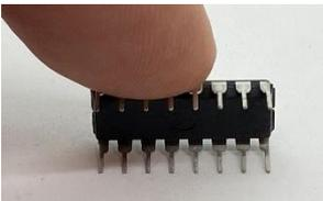
You will also want to make sure the notch at the top of each IC aligns with the DIP socket, and that the correct chip is placed where indicated on the silk screen.
