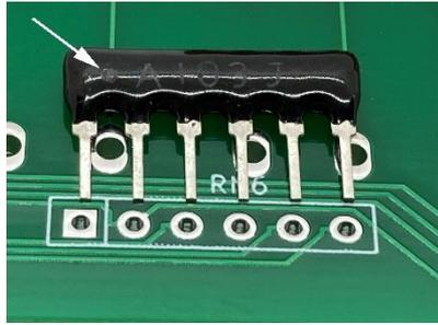
The two 2.2k $\Omega$  yellow resistor arrays are labeled “10X-2-222LF” and are installed in RN1 and RN4. The orientation is not important (they are isolated resistors, not bussed resistor arrays), but I like to install them with the dot to the left for consistency.
