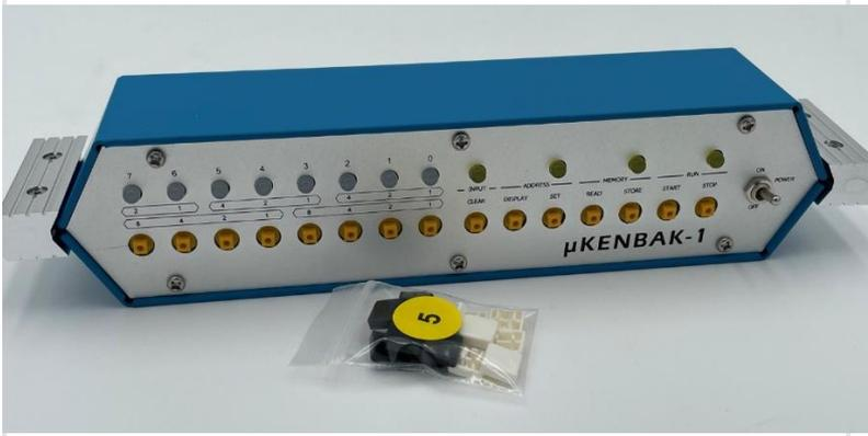
The button caps will fit in any orientation, but I have found that it's best to have the buttons mounted as pictured. It makes it easier to pry the buttons off (from the top and bottom) if necessary.
