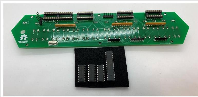
You'll notice the legs on the ICs are typically bent outwards just a bit. You will need to make the legs perpendicular to the body. There are IC insertion tools that do that, but I like to simply push down on a flat surface to align them.
