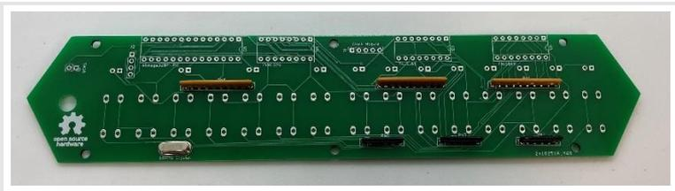
Add the DIP sockets to the back side of the printed circuit board (the side with the “Open Source Hardware” logo.)
