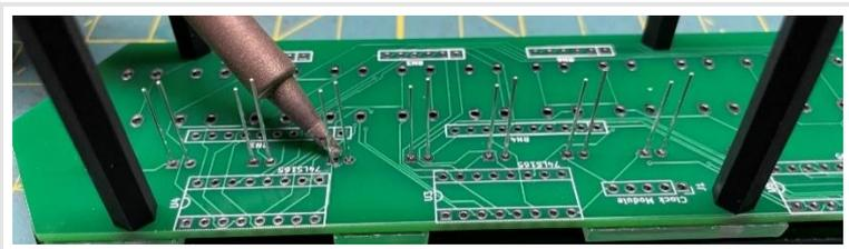
Remove the faceplate and add the tactile switches in place, make sure they are aligned.
