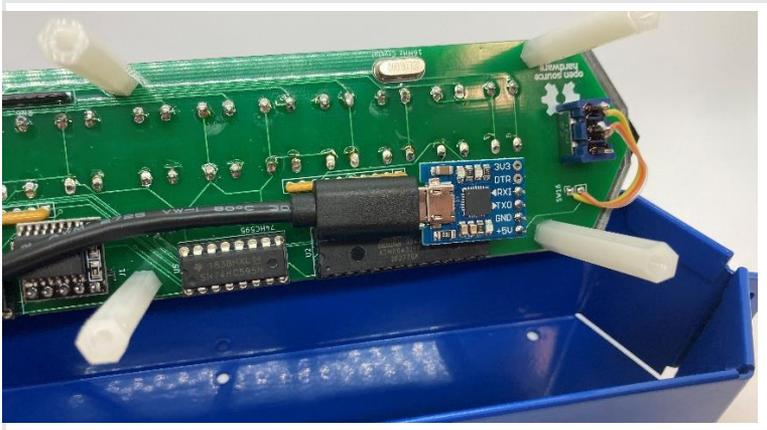
And secure the circuit board and front panel to the case with six 8mm bolts.
