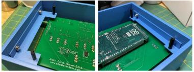
Plug the USB extension cable into the Programming Port on the Arduino Due (the port closest to the power jack.)
