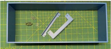
Place the aluminum frame with the holes closest to the top, and mount the smaller side bracket **exactly as shown**:
