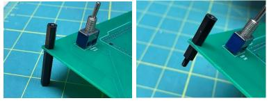
Place the assembled main circuit board in place, directing the 8mm standoffs into the mounting holes.
