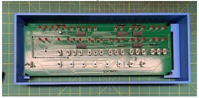
Secure the board in place with four 20mm nylon standoffs:
