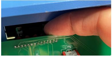
Secure the rear panel in place with your existing nylon bolts.
