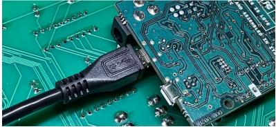
This step is optional. The small expansion circuit board is just a couple millimeters too tall for the new case. You can leave it as is if the rear panel sitting at a slight angle on the back of the case does not bother you. Otherwise you can take a pair of side-cutters and snip a small piece off the expansion board. There are no traces in this part of the circuit board, and I have cut several of these with no problems.
