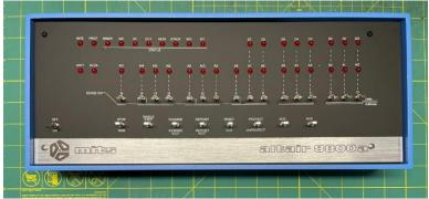
You may have to push a few of the toggles to the side to get the panel in place. When it is in correctly, the toggles will stick out like this:
