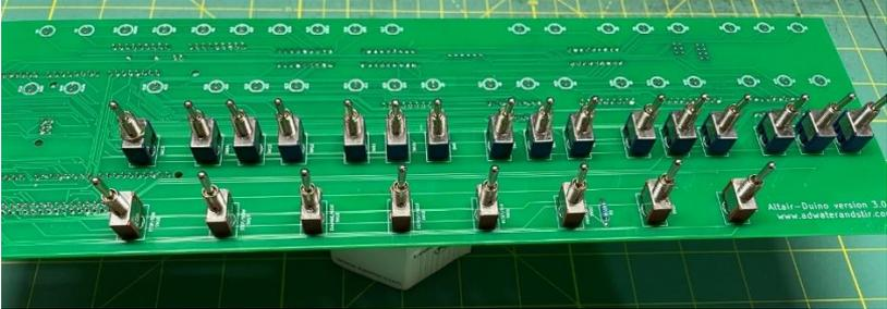
The MTS-123 (three-way momentary) switches will fit a bit tighter than the MTS-102 switches. You can get them in place by rocking them side-to-side, or you can gently squeeze the lugs a bit toward the center.
