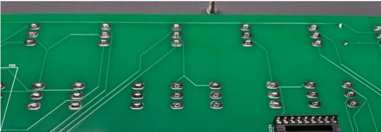
I like to support the front panel from the sides and the middle. Solder the switches in place. You may have to press up on each switch as you solder the first lug in place to make sure it is firmly in place.
