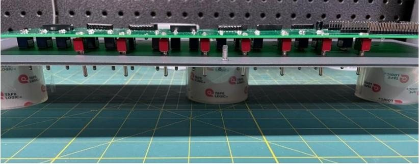
Be careful that you don't over-heat the toggle switches while soldering. This can damage the switch mechanism. Instead of soldering all three lugs on the toggle one after the other, I solder the top lugs on all switches, then the center lugs, then the bottom lugs like this:
