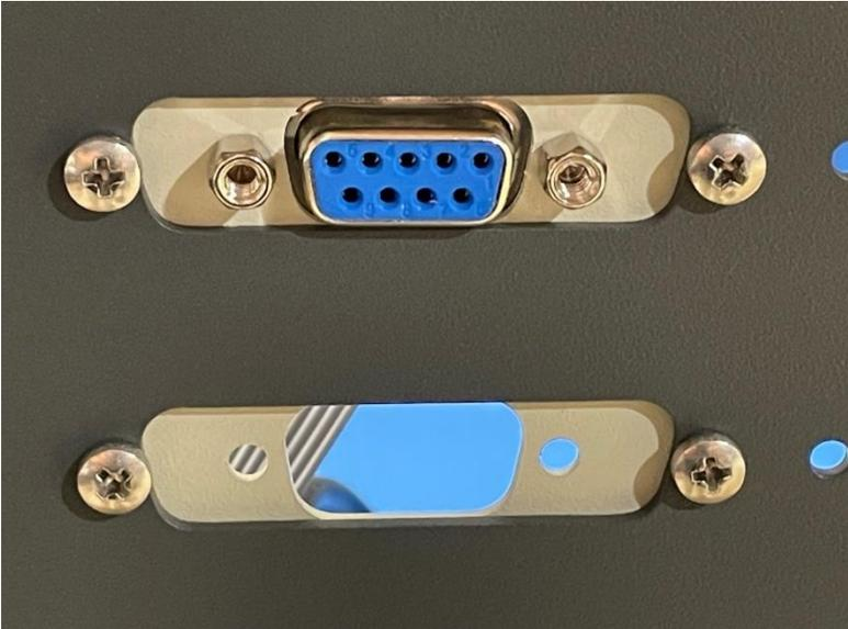
Plug the DE9 port into the expansion board with the red stripe toward the audio connection.
