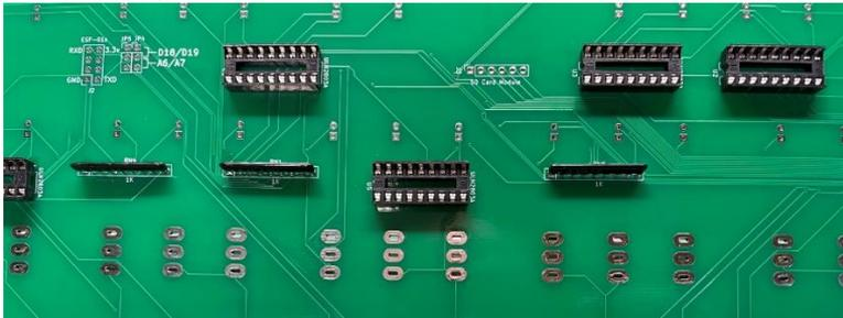
We're going to use the Arduino Due to hold the pin headers temporarily while we solder them to the main circuit board. Cut (or locate) the following segments:
