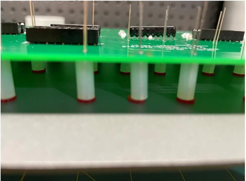
You may have to press down on the circuit board as you solder each leg of the LEDs. As you do this, make sure the long lead is in the correct location.
