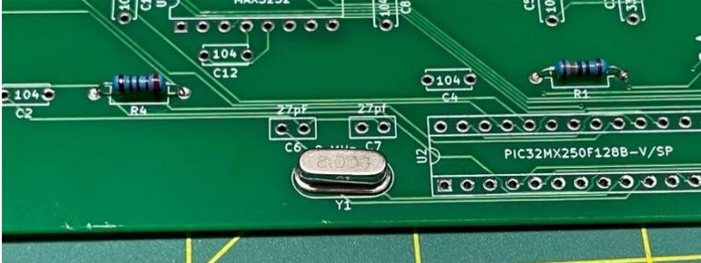
Add the DIP sockets (from bag 2) and two 27pF capacitors and nine 100nf (104) capacitors. You may notice there are locations for ten 104 capacitors. The 104 and 334 capacitors by the location of the voltage regulator will be added later.
