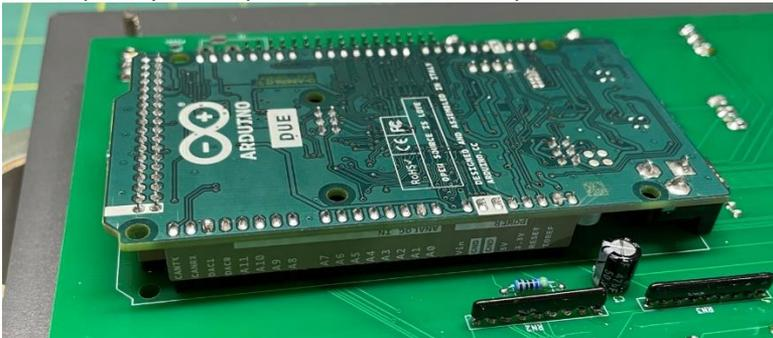
This is a good time to test your Altair-Duino. Plug a micro USB cable into your Arduino and connect it to a computer (or other USB power supply.) Try launching Kill-the-Bit by setting SW1 up and lower AUX1 as seen in this video: [adwaterandstir.com/FirstTest](http://adwaterandstir.com/FirstTest).
