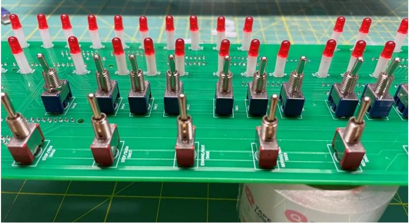
When all 36 LEDs are in place, put the front panel in place and flip the board over, placing it on your supports.
