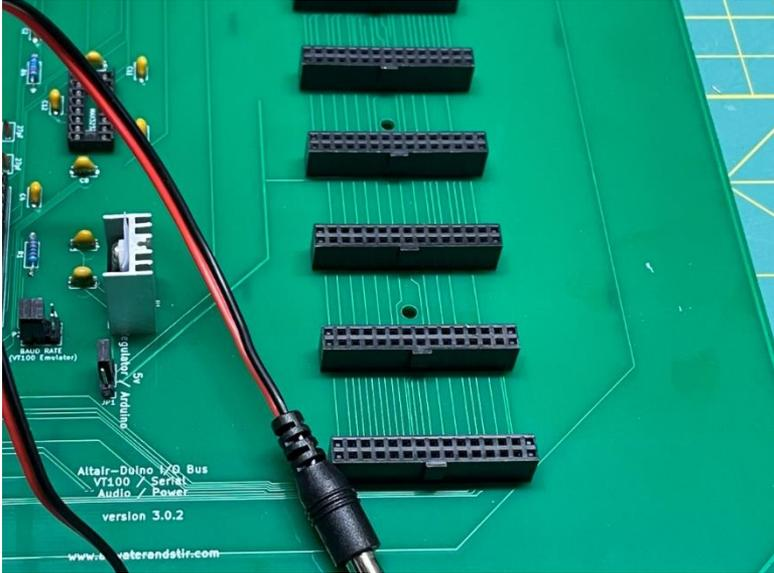
Finally, add the PIC32 microprocessor and SP3232 from bag 5, and your expansion board is complete.
