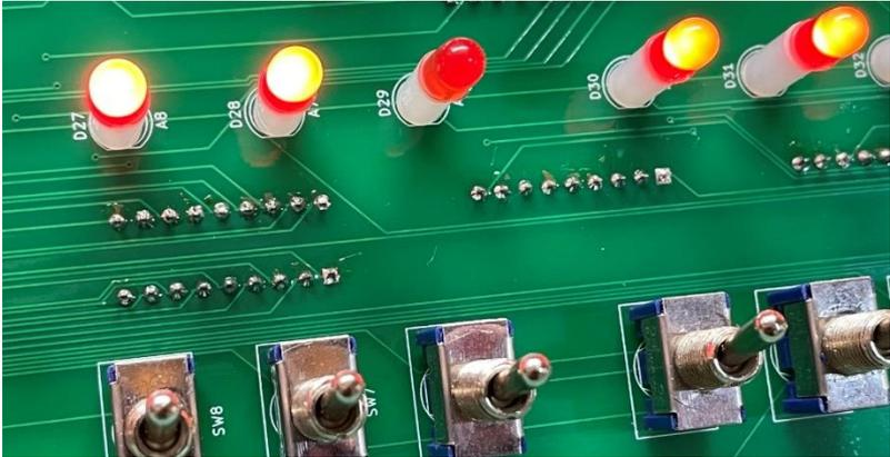
I checked the solder connections and all looked good. One thing I have seen in the past is that the toggle switches may develop some oxidation on the contacts when in storage. If you run into this situation, just toggle the switch back and forth several times quickly and try again. That was my problem in this case:
