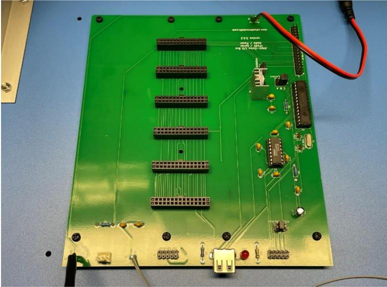
Attach the USB-A extension cable to the rear panel. The cable comes with two bolts, but I like to use one of the bolts that came with the cable, and the other bolt remaining in bag 6 (so it matches the others around the port panel).
