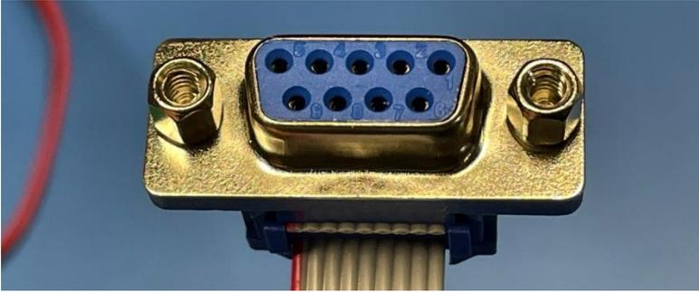
Mount the connector in the top port on the rear panel and replace the jack screws.
