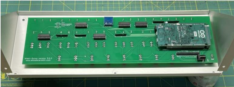
Hold the front panel in place and secure it with several toggle switch lock washers and nuts (that you previously removed from the switches). You can use an 8mm socket driver for this.
