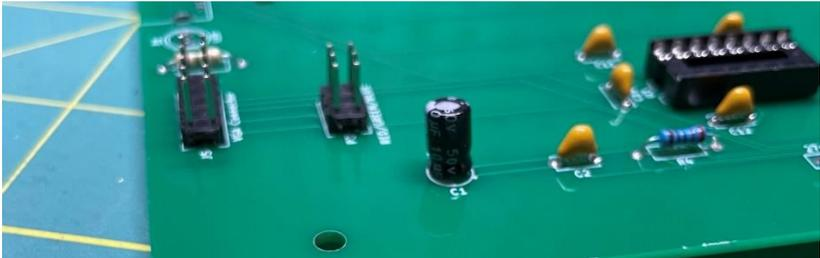
Add the USB-A jack and 3-pin fan connector to the circuit board as shown. Be sure to position the 3-pin connector with the correct orientation. Also add an LED next to the USB-A jack. Pay attention to the polarity (flat side indicated on silkscreen).
