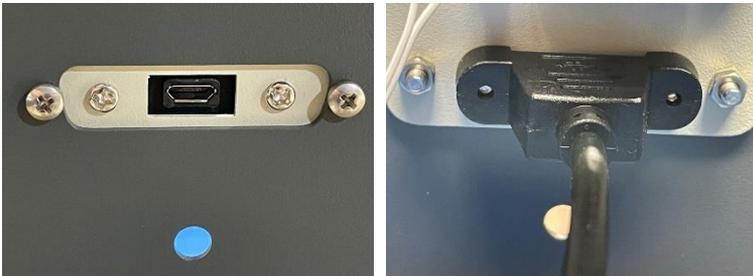
This would be a good time to add the front panel assembly and bracket back into the case. Secure it with four M4 bolts and four M4 nuts.
