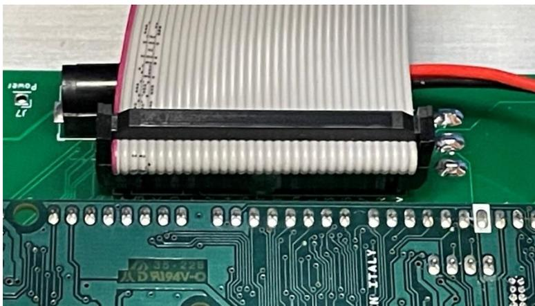
Plug the other end of the cable into the expansion circuit board.
