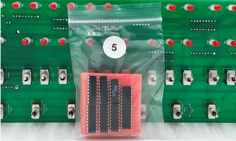
Insert five ULN2803 chips in the five 20-pin DIP sockets on the main circuit board. Be sure to pay attention to the orientation notch.
