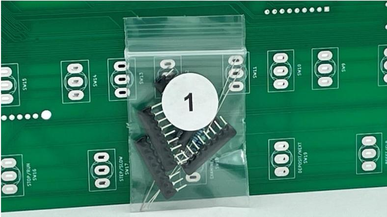
Add the five resistor arrays in RN1-RN5 on the back of the circuit board (look for screen print outlines), making sure the dot indicator faces to the left side (where the square is on the circuit board) as pictured.
