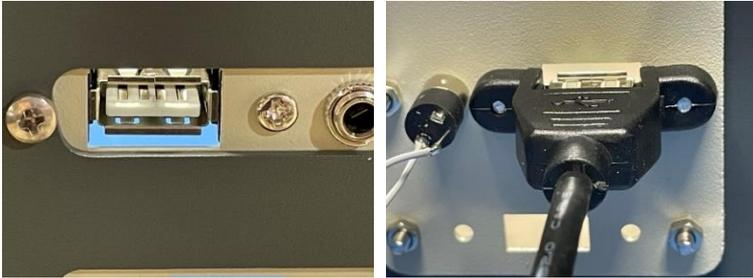
Plug the other end into the USB-A on the expansion board.
