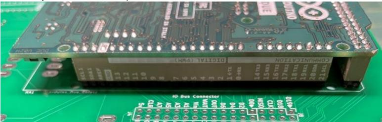
Solder all header pins in place (note: this is where most errors happen – it’s easy to miss one or two header connections.)
