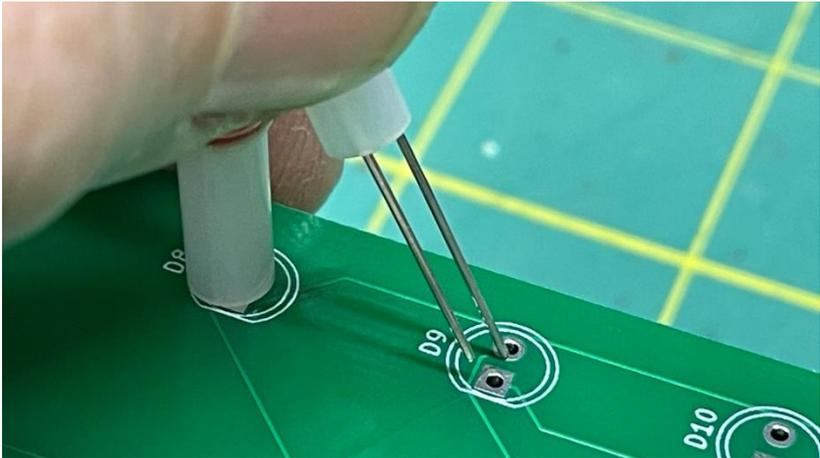
I like to support the circuit board at both ends and one support in the middle.
