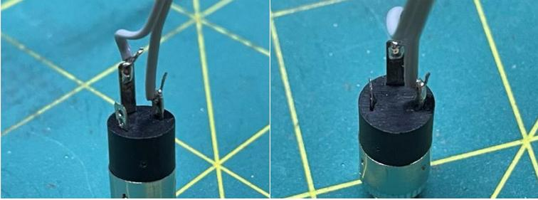
Get the DC-022 power connector and the length of power cable with an XH connector already attached and solder it to the power connector as shown:
