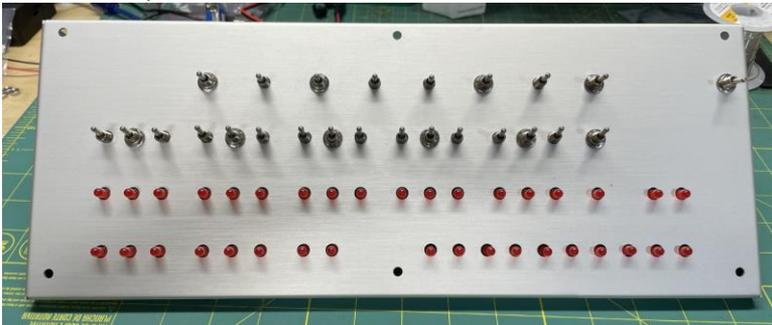
You don't need to secure every switch, just enough to keep the board in place (you can see in the photo I secured 11).
