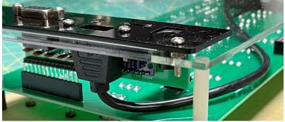
Secure the clear panel to the 28mm standoffs with four 8mm M3 bolts.
