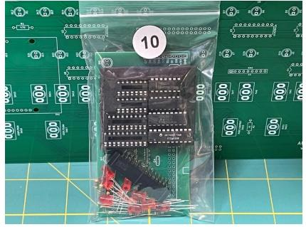
Start with the resistors. All eight resistors are  $150\Omega$ .
