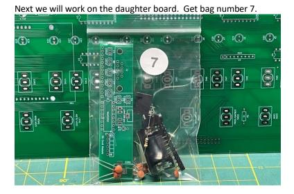
Start by installing the seven capacitors. These ceramic capacitors are not polarized, so orientation is not important.
