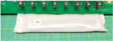
Insert five ULN2803 chips in the five 20-pin DIP sockets on the main circuit board.
