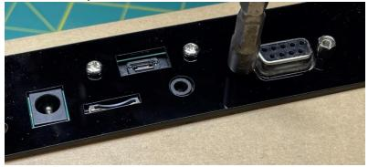
Plug the USB extension cable into the Programming Port on the Arduino Due (the port closest to the power jack.)
