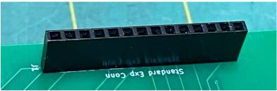
We're going to use the Arduino Due to hold the pin headers temporarily while we solder them to the main circuit board. Cut (or locate) the following segments:
