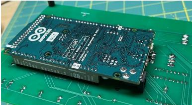
This is a good time to test your Altair-Duino. Plug a micro USB cable into your Arduino and connect it to a computer (or other USB power supply.) Try launching Kill-the-Bit by setting SW1 up and lower AUX1 as seen in this video: adwaterandstir.com/FirstTest. Next, set SW0 through SW15 up and lower EXAMINE and see if all address LEDs illuminate. If not, check your solder connections.
