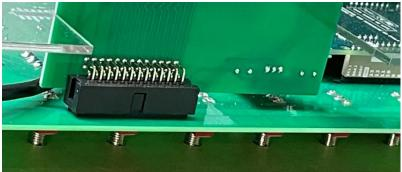
You can attach the expansion bus board to the L-brackets with the  $\ensuremath{\mathscr{V}}^{\prime\prime}$  bolts from below.
