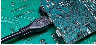
Insert the 14-pin male header into the 14-pin female header, and route the USB extension cable as shown.
