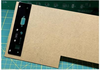
Remove the jack nuts from the DE9 connector. You can do this with a 3/16'' driver or a pliers.
