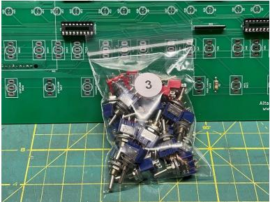
I like to first add the 17 on-off toggles and hold them in place with the front panel while soldering. This ensures the toggles switches remain in alignment with the front panel. Next, add the 8 on-off-on toggles and again hold them in place with the front panel while soldering.
