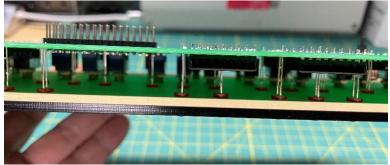
Then support the front panel while you solder the LEDs in place.
