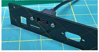
Take the clear acrylic pane and peel the protective paper. **I'm going to leave it on so it shows up more plainly in a few photos.** Attach the rear ports panel with two 8mm M3 bolts and two nuts as shown in the photo.
