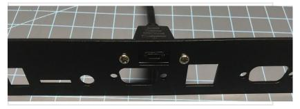
Remove the jack screws from the VGA and Serial connectors with a needle-nose pliers, or a 3/16" or 5mm socket.
