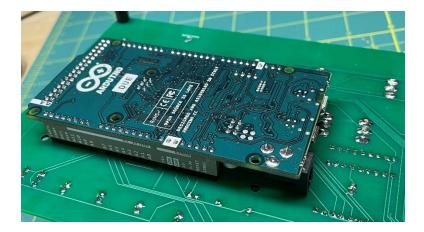
This is a good time to test your Altair-Duino. Plug a micro USB cable into your Arduino and connect it to a computer (or other USB power supply.) Try launching Kill-the-Bit by setting SW1 up and raise AUX1 as seen in this video: adwaterandstir.com/FirstTest. Next, set SW0 through SW15 up and lower EXAMINE and see if all address LEDs illuminate. If not, check your solder connections.
